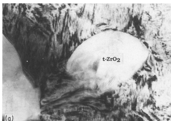
Figure 7 Transmission electron micrograph showing incorporation of a t-grain into a tweed grain: (a) bright-field image, (b) dark-field image ( g = \{2\ 1\ 1\} ), same specimen as Fig. 6.
